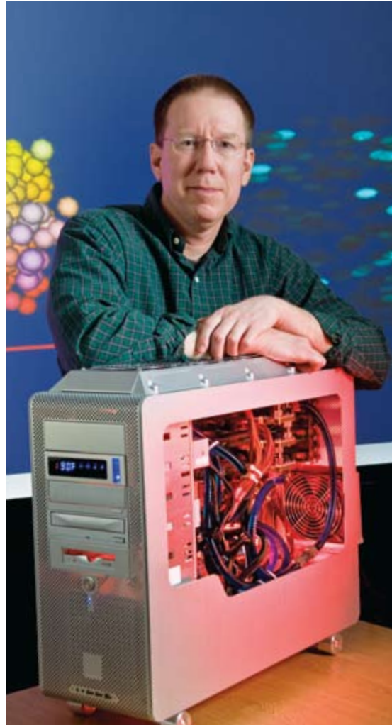
Dr. Jack Collins displays a computer system he developed for the National Cancer Institute that uses a series of graphic processors for tackling drug design problems, such as screening hundreds of thousands of candidate drug molecules. Each candidate drug now can be screened in minutes instead of the hour it used to take using a more expensive computer cluster.
