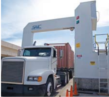
Another version of SAIC's VACIS, the P7500 inspection system, scans up to 150 cargo containers per hour.
