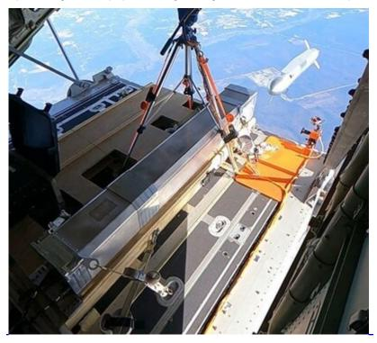
Store separation testing from an AC-130J, conducted in December 2023, confirmed digital twin predictions of safe separation, benign store dynamics, and trajectory characteristics. Additional captive flight testing demonstrated integration with the NSWC Battle Management System (BMS), operational flight software function, navigation performance, and flight safety system functionality.
